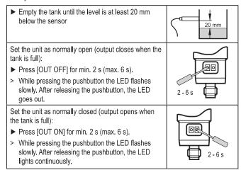
The unit is now ready for operation. For the detection of media with a low dielectric constant (e.g. plastic granulates or oils) no further setting is required.
