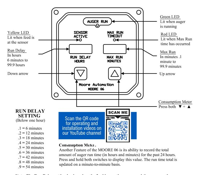
Note: The Run Delay setting begins when the feed leaves the sensor and the sensor active light is off. This feed line control is designed to start immediately when the power is on. Pressing the up or down arrow keys at any time will stop the current status and go into run delay.
